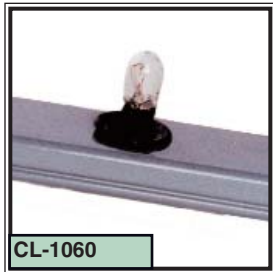
CHANNELITER (6) LO194 2.4W Wedge Base Phosphatized Steel Spacing: 10" on Center
